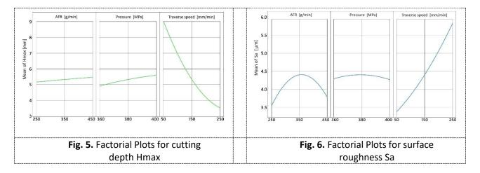
This corresponds to a set of the following control parameters: abrasive flow equal to 450 g/min, working pressure equal to 380 MPa, and traverse speed equal to 50 mm/min. Under these levels of control parameters, the output parameters were equal appropriately: cutting depth Hmax = 9.02 mm and surface roughness Sa = 3.01  $\mu$ m.
