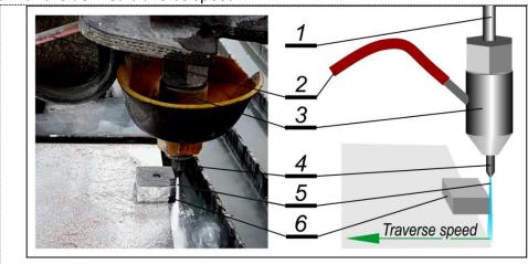
**Fig. 1.** Real view and schematic of AWJ cutting process: 1-water inlet, 2-abrasive inlet, 3-cutting head, 4-focusing tube, 5-AWJ, 6-target material
