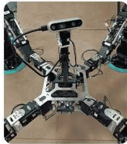
(a) Quadruped Robot with 3D Flexible Legs Fig. 2. (a) Quadruped robot with 3D flexible legs demonstrating adaptive surface conformity [8]. (b) Four-legged robotic organism inspired by biological locomotion for enhanced climbing agility [9].
